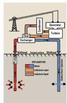
Diagram showing how electricity is generated from a hot-water hydrothermal system. The part of the hydrothermal water that flashes to steam is separated and used to drive a turbine generator. Wastewater from separator and condenser is injected back into the subsurface to help extend the useful life of the hydrothermal system.
