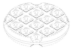
In this second design patent, only the dimples—not the outer contour—are shown in solid lines. That means that only the dimples are claimed. The second patent would also be infringed by a circular potato product with more dimples, as long as this set of dimples was a visual match for the claimed design. So the second patent is much broader than the first.
