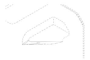
Because design patent claims only cover what is shown in solid lines, this claim only covers the small plane shown in the bottom left of this closer view.<sup>43</sup> So it would be infringed by any rechargeable battery that included that plane, regardless of what the rest of the battery looked like.
